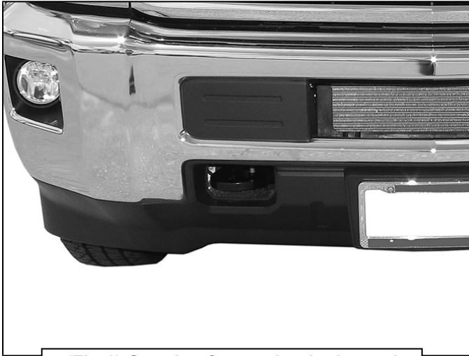
(Fig 1) Opening for tow hook pictured
