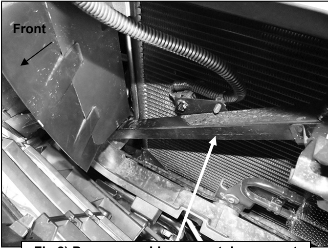
Fig 8) Passenger side square tube support between grille and radiator pictured
