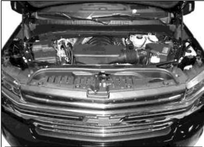
(Fig 12) Remove plastic cover from top of grille
