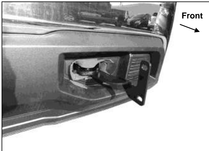
(Fig 11) Driver/left Bracket assembly installed
