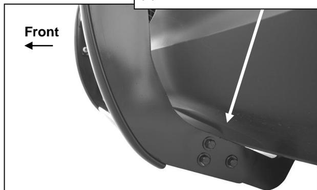
**(Fig 7) Attach Grille Guard to Frame Brackets**
