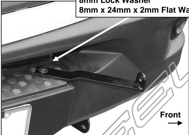
**(Fig 6) Attach driver/left Center Bracket to bumper**
