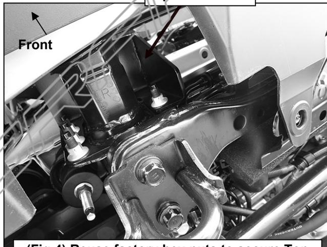
(Fig 3B) Passenger side Top Bracket pictured
