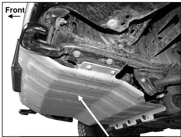
**(Fig 4) Remove skid plate if equipped**
