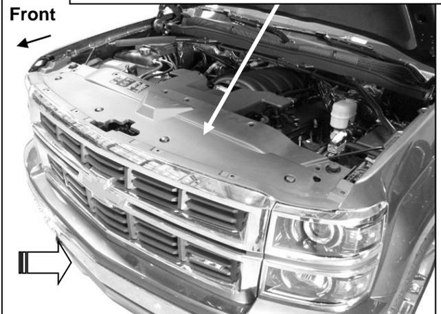
**(Fig 2) 2014-15 models, from behind bumper, release clips and hardware attaching plastic fascia panel (arrow) to top of bumper and fender. Remove fascia panel to access bumper hardware from above.**
