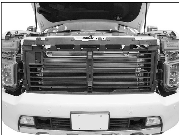
(Fig 7) Grille and fascia removed
