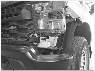
(Fig 4) Remove fascia body panel
