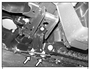
(Fig 8) Remove bolts attaching bottom of bumper to brackets (arrows). Driver/left side pictured
