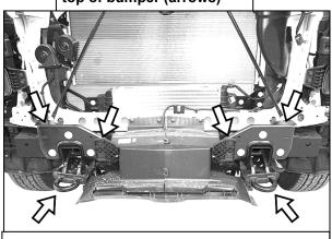
(Fig 11) Remove bumper brackets and tow hooks if equipped. Models with turbo, unplug harness and remove shroud and shutter assembly
