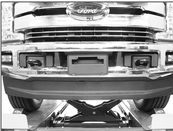
(Fig 3) Remove plastic air dam from bumper
