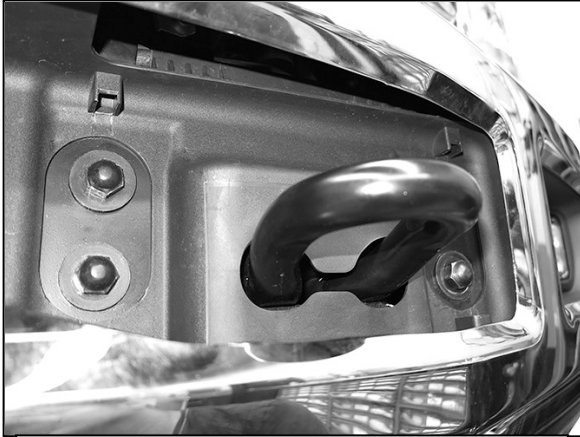
(Fig 6) Remove bumper bolts from front
