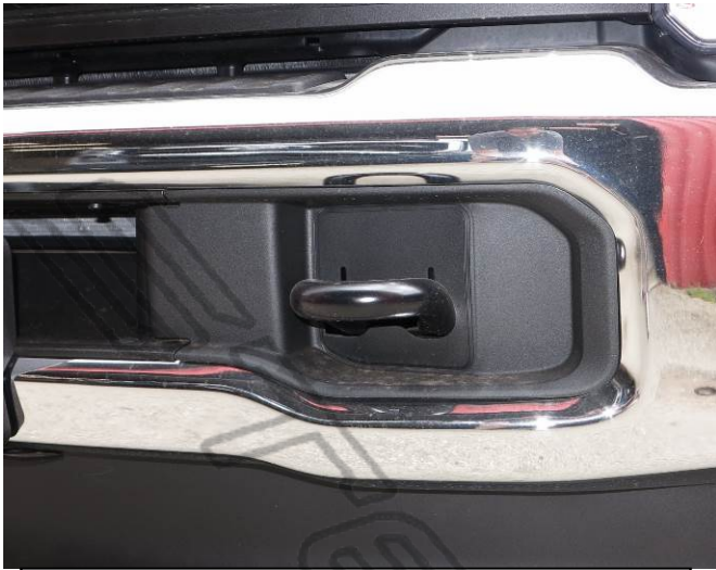
(Fig 3) Remove plastic cover around tow hook
