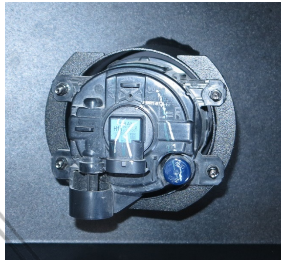
(Fig 12) Attach fog lights to bumper using 4mm hardware
