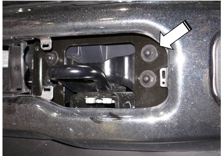
(Fig 4) Remove bumper bolts (driver side pictured)
