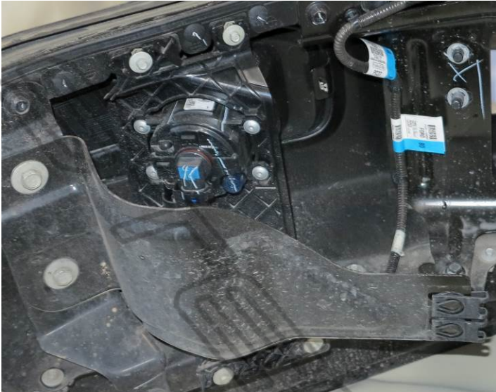
(Fig 11) Unplug and remove fog lights from OE bumper (if equipped)
