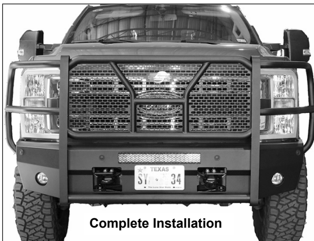
(Fig 21) Remove center screen if equipped with grille mounted camera. Push Plastic Plugs into holes in Bumper for license plate
