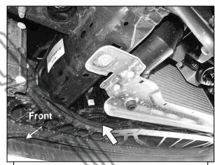
(Fig 4) Hybrid Models Only, locate alert speaker behind driver/left side of bumper
