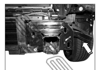
(Fig 6) Remove bumper. Also remove the factory frame extension (arrow-optional)
