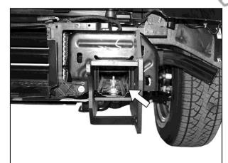
(Fig 8) Driver/left Frame Mounting Bracket attached to inner Double Nut Plate (arrow)
