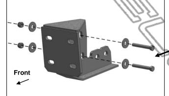
(Fig 5) Attach passenger/right side Frame Bracket to outside of frame
