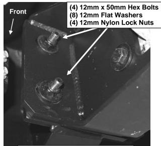
(Fig 9) Attach passenger/right side of Bumper to Frame Bracket
