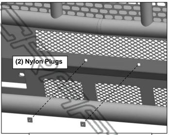
(Fig 11) Push Plastic Plugs into holes in Bumper to attach license plate
