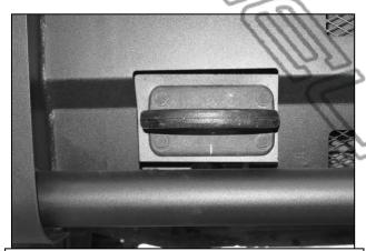
(Fig 10) Reuse factory hardware to attach the tow hook to the mounting location in the Bumper
