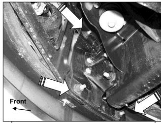
(Fig 1) Remove hex nuts (arrows) to remove bumper from bumper brackets
