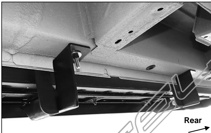
(Fig 21) Passenger side Bracket layout w-Support Brackets
