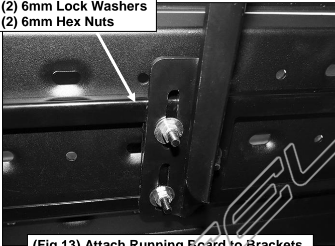
(Fig 13) Attach Running Board to Brackets
