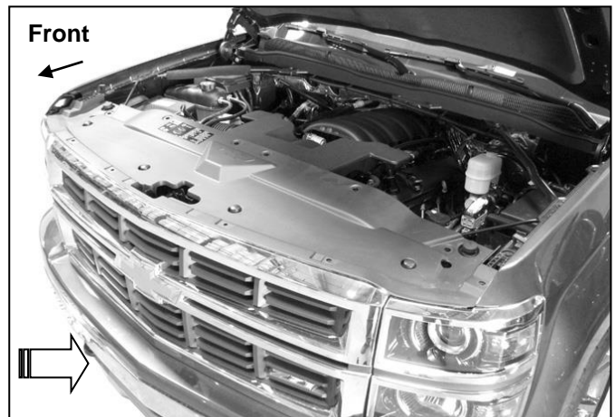
(Fig 2) On 14-15 models, from behind bumper, release clips and hardware attaching plastic fascia panel (arrow) to top of bumper and fender. Remove fascia panel to access grille and bumper hardware from above.
