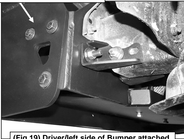
(Fig 19) Driver/left side of Bumper attached to Winch Tray Bracket Assembly
