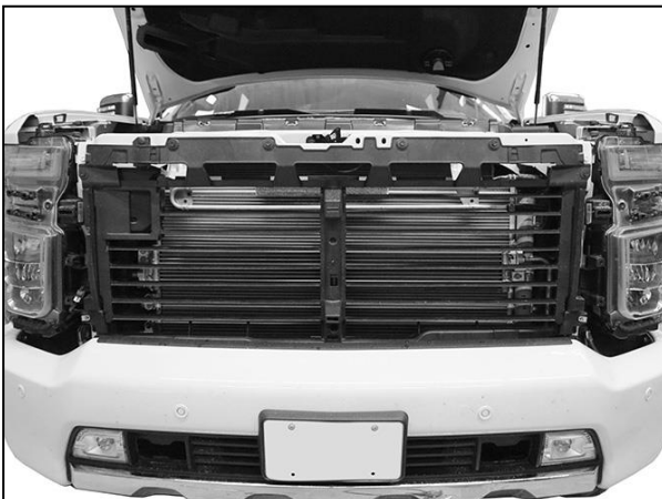
(Fig 7) Grille and fascia removed
