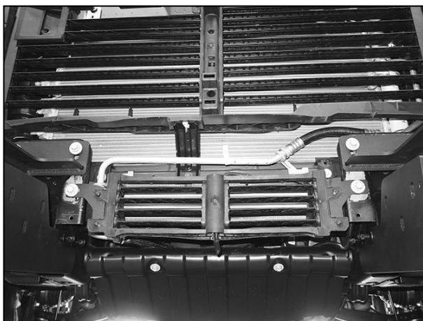
(Fig 17) Attach shutter assembly, (if equipped), to front of Relocation Brackets
