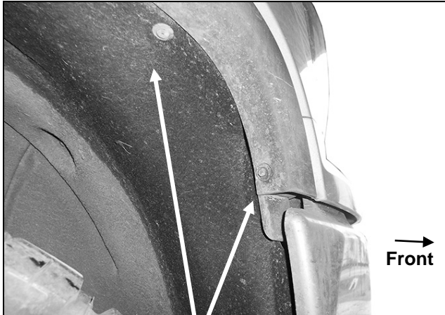
(Fig 1) Release clips and hardware attaching fender liner and front end of flare (arrows)
