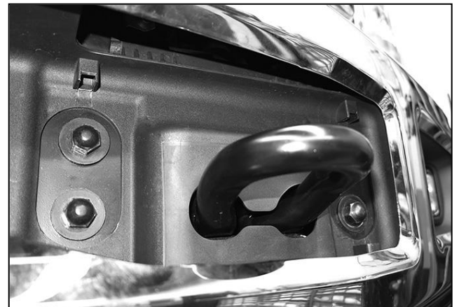
(Fig 6) Remove bumper bolts (driver side pictured)
