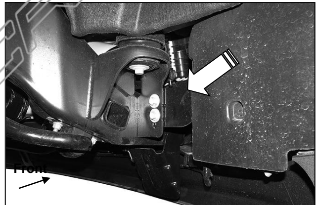
(Fig 4) Remove outer bumper support brackets between frame and bumper (arrow)
