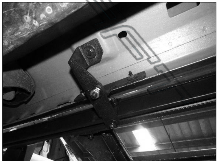
(Fig 20) Universal Mounting Tube attached to the Center Mounting Bracket.
