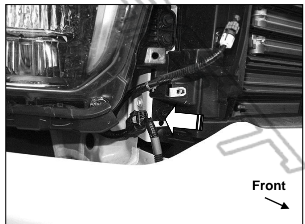
(Fig 8) Disconnect all wire harnesses leading to front bumper
