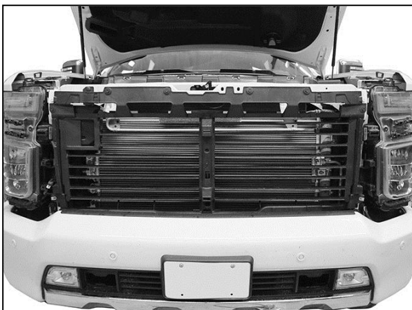
(Fig 7) Grille and fascia removed
