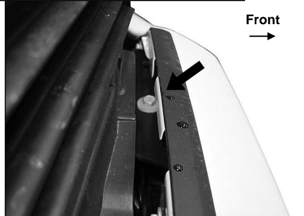
(Fig 10) From above, remove the hex bolts attaching the bumper assembly to the frame bumper brackets (top visible-arrow)
