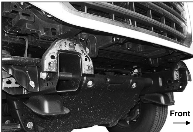
(Fig 11) Remove bumper brackets and tow hooks, reinstall plastic grille and fascia panel
