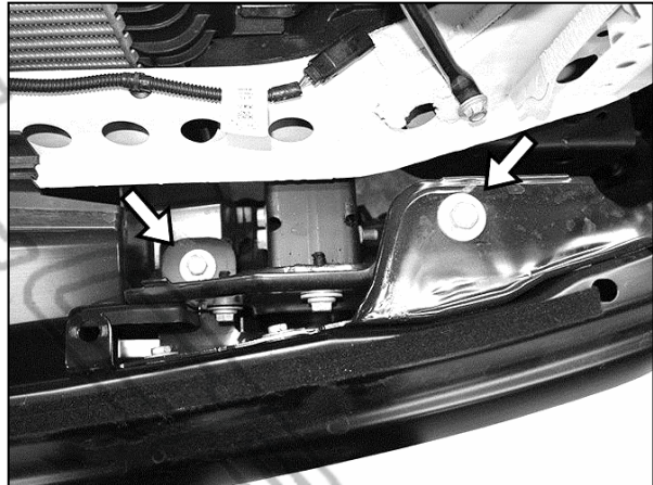
(Fig 10) Remove driver/left top bumper bolts (arrows)
