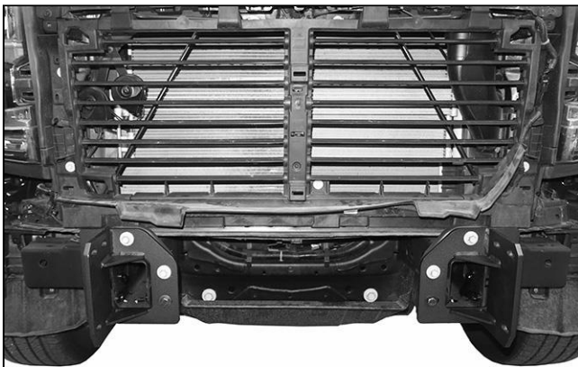
(Fig 21) Complete installation of Frame Brackets
