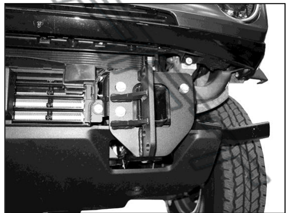
(Fig 8) Driver/left side Bracket installed
