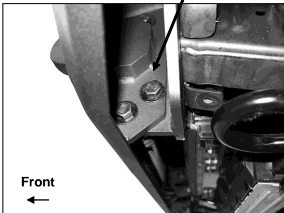
(Fig 19) Driver/left side of Bumper attached to Double Bolt Plate pictured from below
