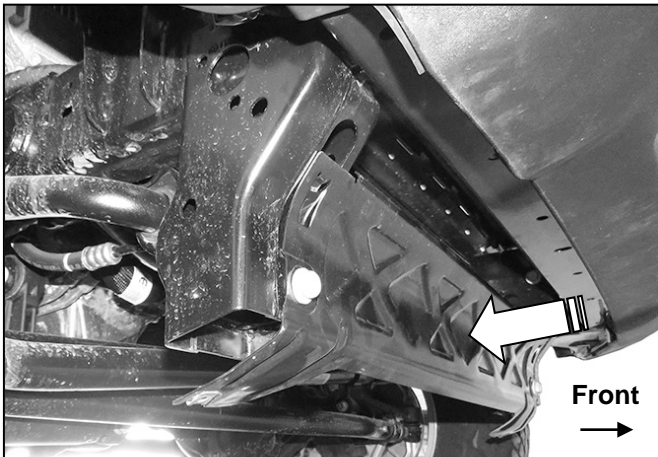
(Fig 1) Remove splash guard and bracket (arrow)
