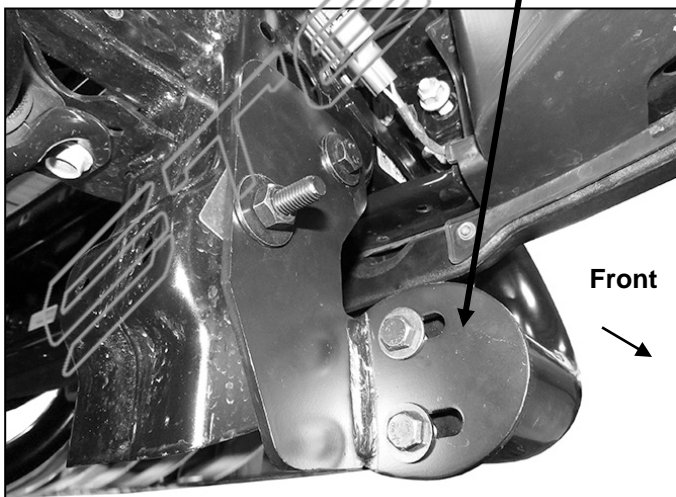
(Fig 7) Attach end of Bull Bar to passenger/right Mounting Bracket. Pictured without splash guard for instruction purposes only
