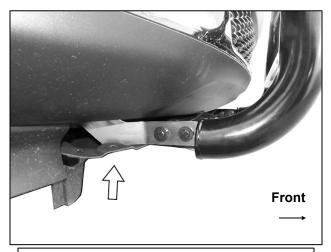
(Fig 6) Hold splash guard up to bottom of the Brackets. Cut slots in splash guard to clear the Brackets. Reinstall the splash guard
