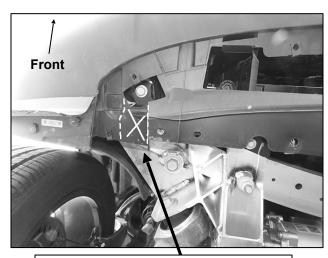
(Fig 3) Cut section from bumper cover to clear the Mounting Bracket
