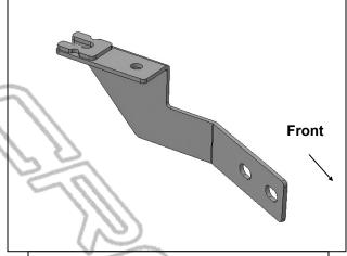
(Fig 2) Passenger/right Mounting Bracket
