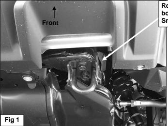
Remove (2) factory hex bolts to remove tow hook. Small tow hook pictured
