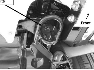
(Fig 4) Driver/left mounting Bracket installation
