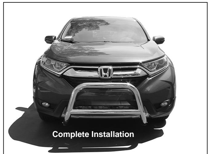
(Fig 10) Complete installation of passenger/right side of Sport Bar pictured without splash guard for instruction purposes only
