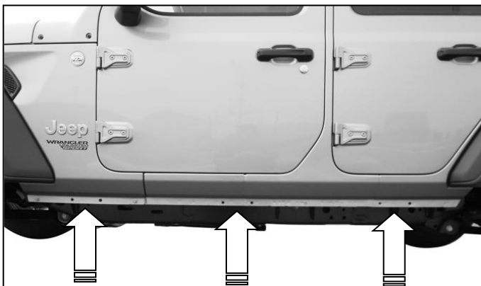
(Fig 1) Locate the (3) factory pair of holes along the pinch weld (Driver/left side pictured)
