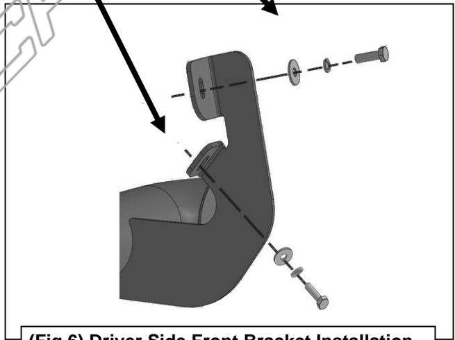
(Fig 6) Driver Side Front Bracket Installation of parts for Vehicle years 2016 and above
