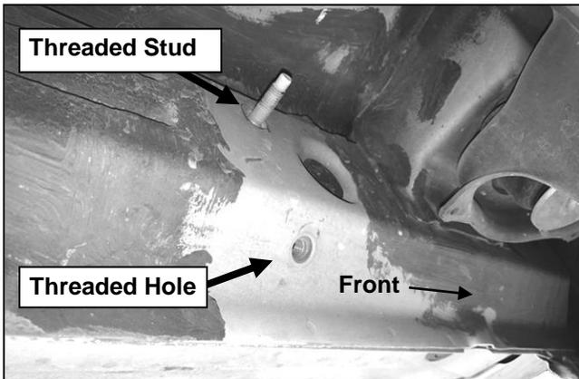
(Fig 1) Driver side Front mounting location pictured. Note: Remove plastic plugs to locate factory threaded holes
