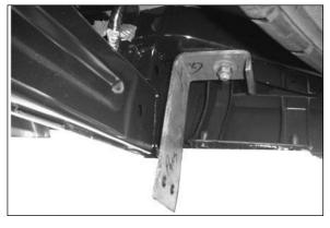
**4.** Fasten bumper bracket to crossmember using (1) 1/2" locknut and (1) 1/2" flatwasher. Tighten until slightly snug. Repeat for opposite side. Passenger side shown.
