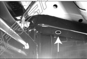
2. Locate (1) hole on each side of the square bumper crossmember. The holes are located between the two bumper brackets that are part of the formed frame rails. Passenger side shown.
