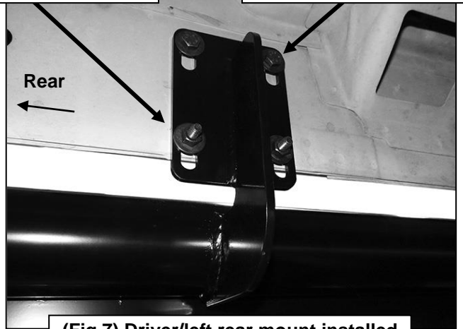
(Fig 7) Driver/left rear mount installed
