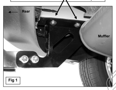
(2) 10-1.25mm x 35mm Fine Thread Hex Bolts (2) 10mm Lock Washers (2) 10mm Flat Washers
