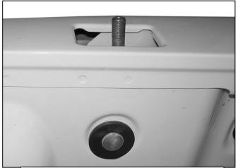
(Fig 5) Use the "J" Bolt to secure the front mounting holes on the Bracket to the stake pocket if possible. Do not drill any mounting holes until after all mounting locations are checked for clearance
