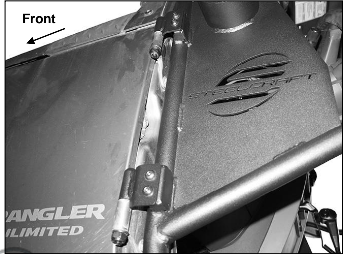
(Fig 8) Door attached to upper and lower hinge assemblies
