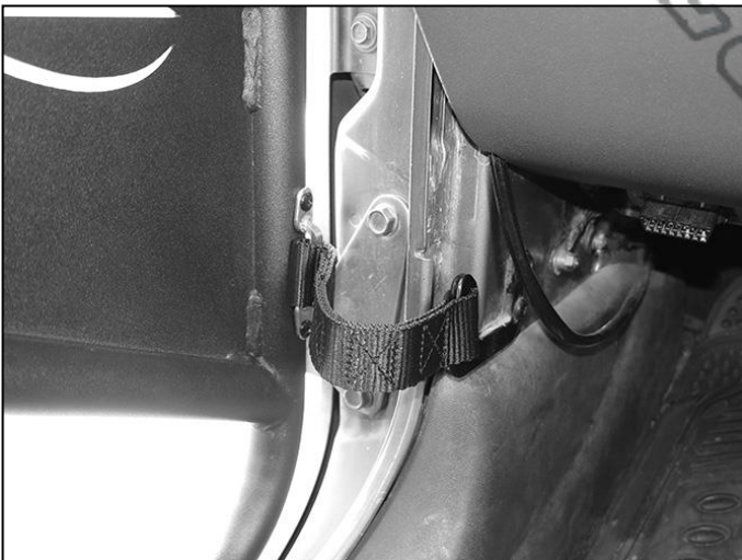
(Fig 9) Slide end of Door Stop Strap over bracket
