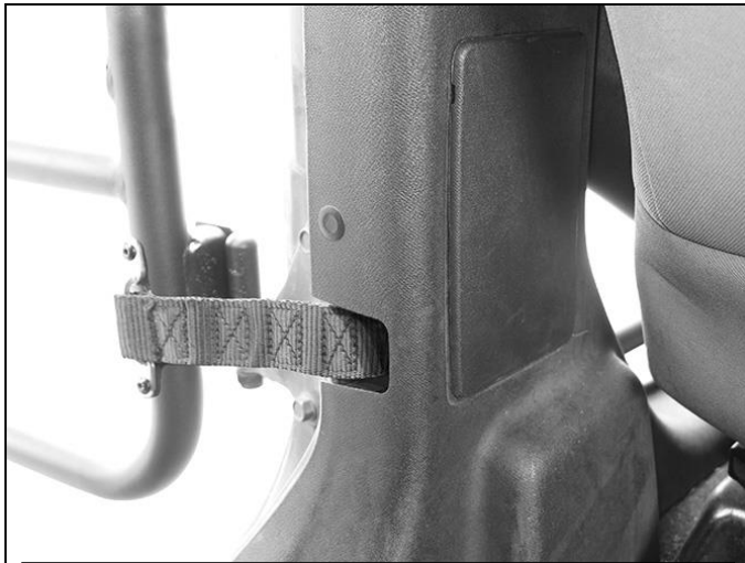
(Fig 9) Attach Door Stop Strap to factory bracket
