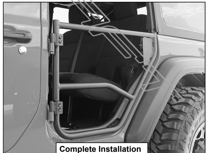
(Fig 11) Adjust Door and Latch assembly for proper operation before fully tightening hardware. Make sure door latch fully closes against striker
