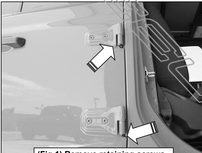
(Fig 1) Remove retaining screws from bottom of hinges (arrows)
