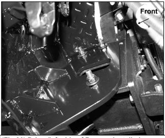
(Fig 26) Driver/left side of Bumper installed
