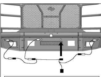
(Fig 29) Reinstall factory wiring harness over Bumper Brackets on back of Bumper. NOTE: Use the included (3) Wire Harness Extensions as necessary to reach the parking sensors
