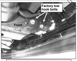
(Fig 11) Remove tow hooks, (if equipped) after bumper has been removed
