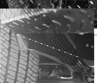
(Fig 30) Trim fender liner flush with bottom of bumper
