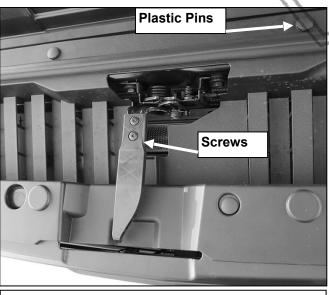
(Fig 5) Remove hood handle and radiator cover
