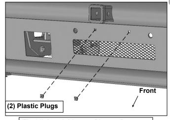
(Fig 31) Attach License Plate to Bumper
