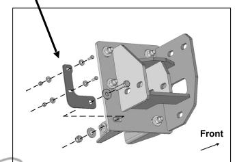
(Fig 20) Attach "L" Relocation Brackets to front of Frame Brackets. Attach shutter assembly, (if equipped), to <u>front</u> of Relocation Brackets
