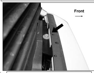
(Fig 10) From above, remove the hex bolts attaching the bumper assembly to the frame bumper brackets (top visible-arrow)
