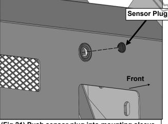
(Fig 21) Push sensor plug into mounting sleeve
