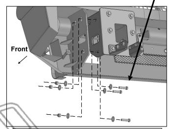
(Fig 25) Attach the Bumper to Frame Brackets
