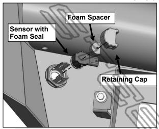
(Fig 24) Insert sensor assembly through the sensor sleeve behind the Bumper
