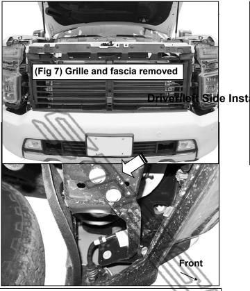
(Fig 9) Remove driver/left and passenger/right outer bumper supports attach to bottom of frame
