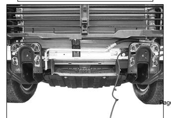
(Fig 8) Disconnect all wire harnesses leading to front bumper
