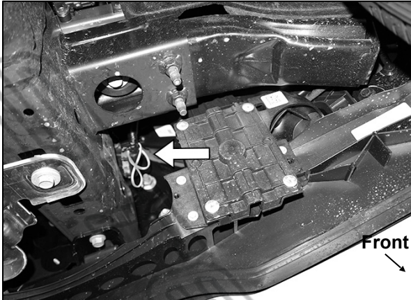
(Fig 3) Locate and unplug main harness plug on passenger/right side of bumper (arrow)
