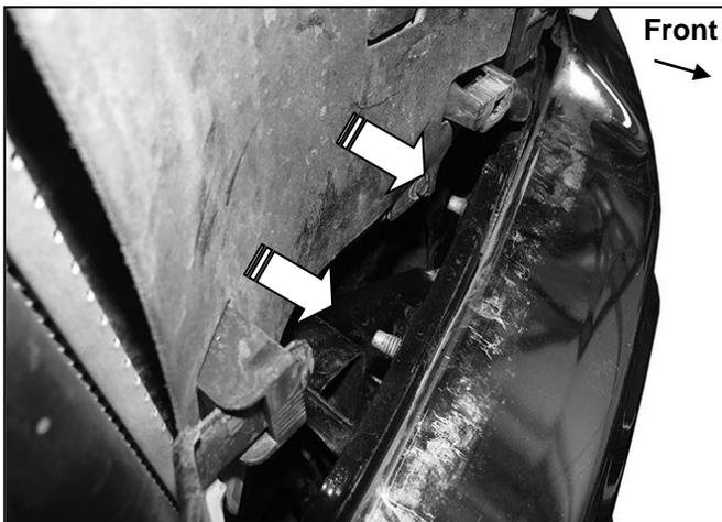
(Fig 3) Remove driver side top bumper hardware
