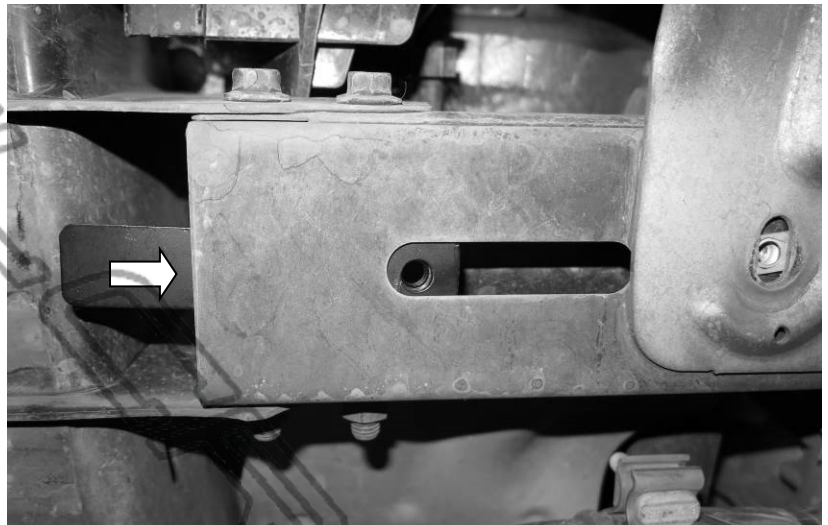
(Fig 7) Insert Nut Plates into open ends of rear crossmember channel. Align hole within slot.
