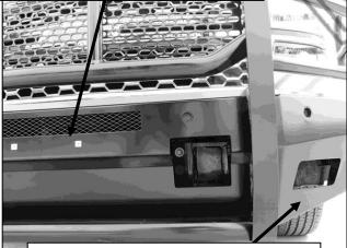
(Fig 22) Push factory fog light into mounting tabs (driver/left side pictured)
