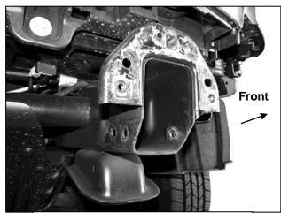
(Fig 8) Remove complete bumper, inner bumper bracket and tow hooks
