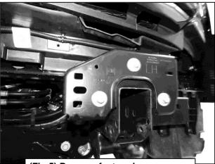
(Fig 5) Remove factory bumper brackets and tow hooks if equipped
