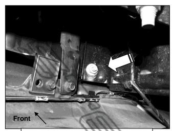
(Fig 3) Remove factory hex nut (arrow) from back of bumper bracket
