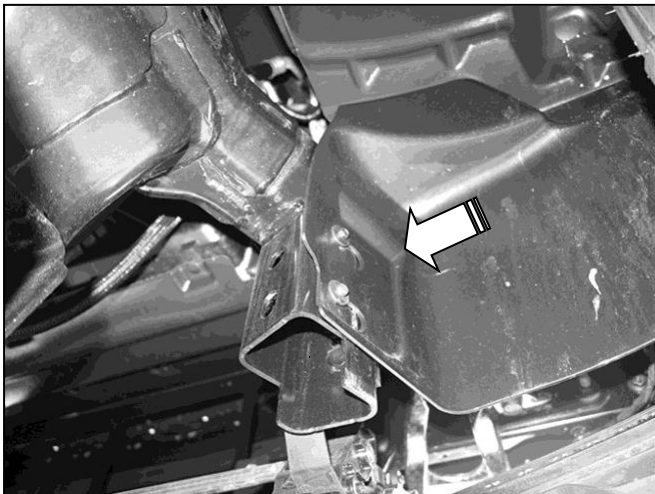
(Fig 1) Remove screws attaching plastic splash guard to frame (arrow). Passenger/right side pictured
