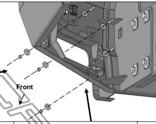
(Fig 10) Attach rectangular fog light to mounting tabs on back of Bumper
