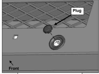
(Fig 6) Models without sensors, insert Plug into Sensor Mount
