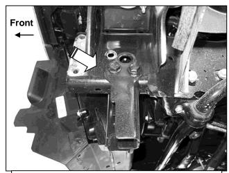
(Fig 2) Remove tow hook and lower frame extensions (arrow) from bottom of the frame
