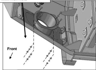
(Fig 13) Attach round fog light to driver/left Adapter Bracket
