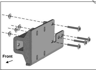
(Fig 3) Reuse factory hardware to attach driver/left Frame Bracket to the outside of frame
