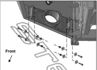
(Fig 12) Reuse hardware to attach round fog light adapter bracket assembly to Bumper
