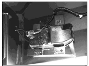
(Fig 11) Attach fog light to mounting tabs on back of Bumper (passenger/right side pictured)
