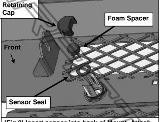
(Fig 8) Insert sensor into back of Mount. Attach Foam Spacer to back of sensor. Snap Retaining Cap onto end of Mount, over sensor and Spacer
