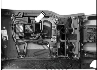
(Fig 5) Disassemble bumper to remove fog light assembly, wiring harness and sensors. Note location of each sensor for reinstallation
