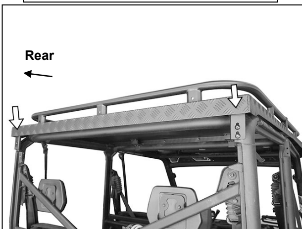
(Fig 14) Reuse the (4) factory bolts to attach rear Brackets on Roof to roll cage (arrows)
