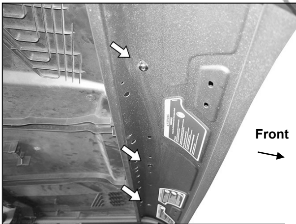
(Fig 3) Remove hardware attaching front of roof to top of roll cage cross panel
