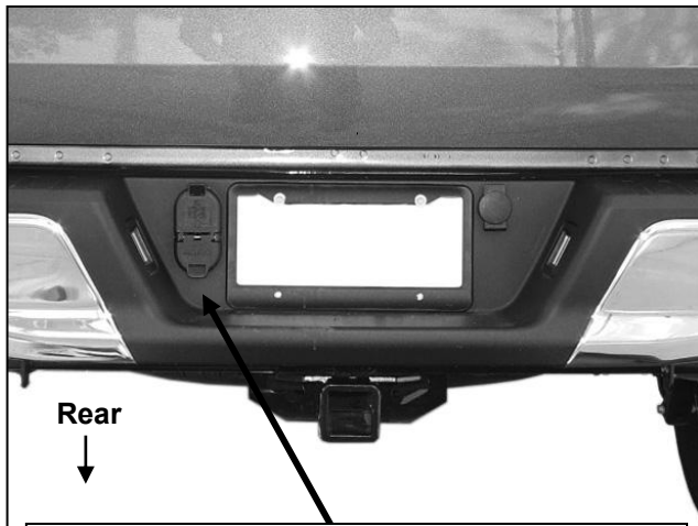
(Fig 1) Unplug and remove 7-wire trailer plug
