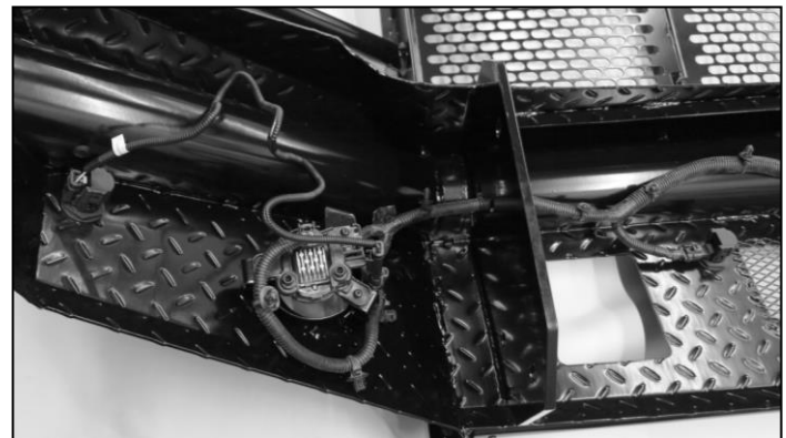
(Fig 24) Use the included (2) Wire Harness Extensions as necessary to reach the parking sensors
