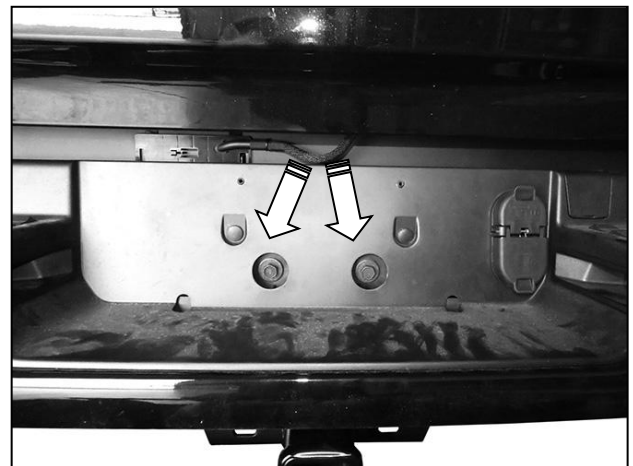
(Fig 2) Remove license plate to access and remove (2) hex bolts (arrows)
