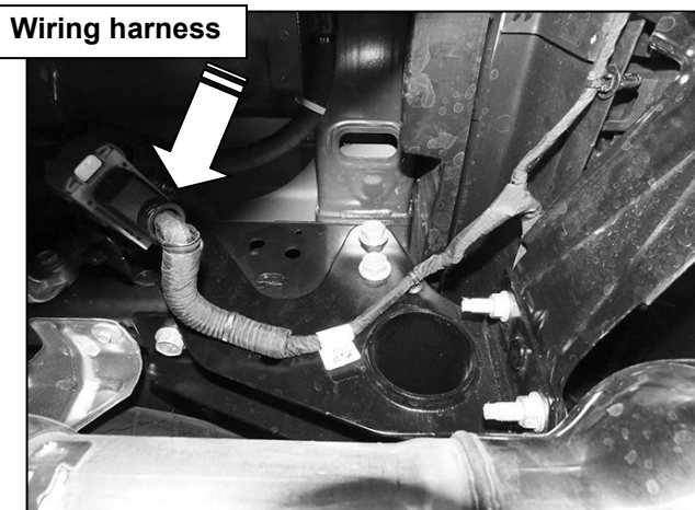
(Fig 1) Unplug wiring harness leading to bumper
