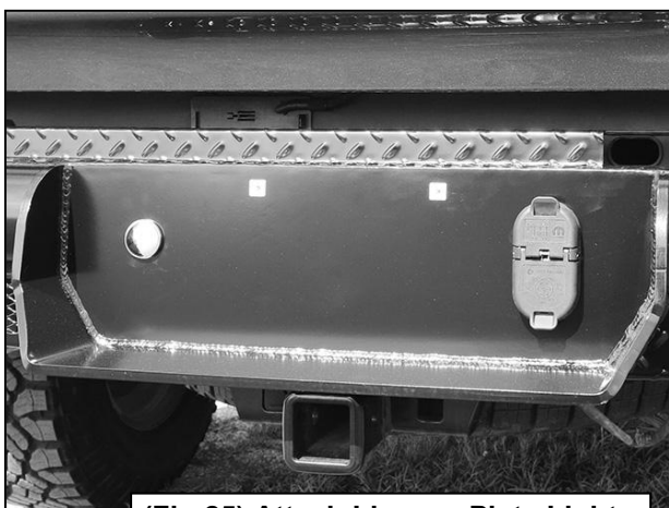
(Fig 25) Attach License Plate Light wire to wiring harness
